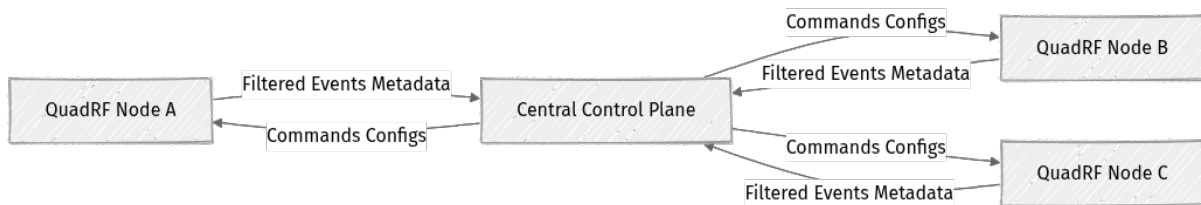
Figure 1: Distributed QuadRF Nodes Reporting Processed Data to a Central Control Plane.
